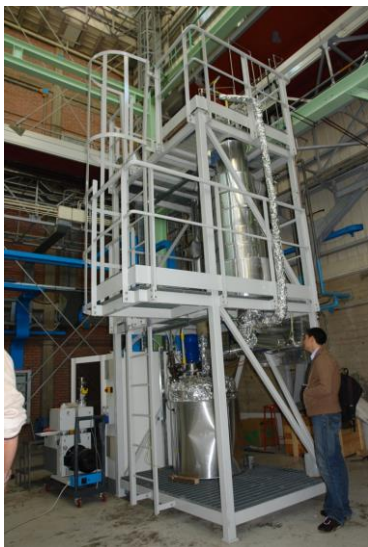
Experimental plant for Tritium extraction (TRIEX)
